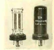
★ New type 5Z4 metal tube —reduced size—no loss in electrical characteristics. Metal shell 3¼ in. x 1 5/16 in. diameter. Filament current reduced to 1.5 amps. Rating of 125 mils with 400 volts (rms) per plate. Will replace octal glass 5Y3 rectifier. Hygrade Sylvania Corp., Emporium, Penna.—RADIO TODAY
